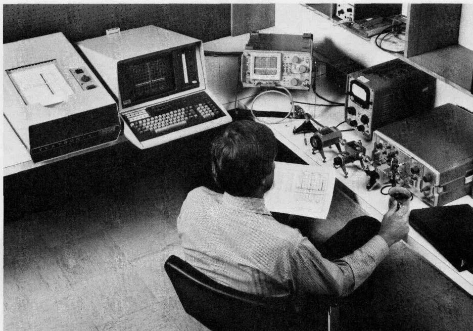
When used with the Tektronix 4052A Graphic Computing System Controller and 4631 Hard Copy Unit, or with the 4662 Digital Plotter, the 492P can provide test results in both graphic and numeric form for the evaluation of microwave signal sources.
